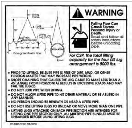
■ Figure 10.12b Lifting lugs for pipes to 8000 lb.
